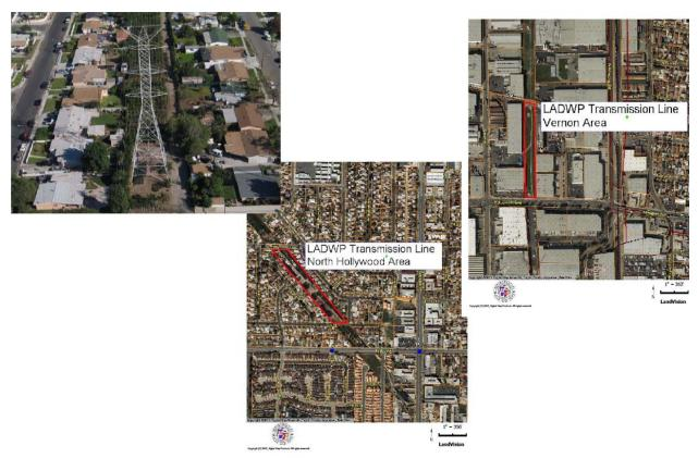
Figure 7 - Examples of how transmission growth is limited by residential and industrial growth along current right of ways
