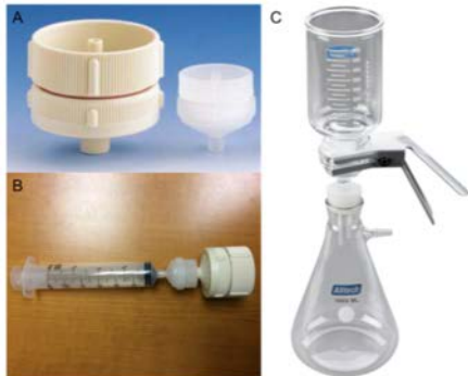
Figure 1. A: 47mm Swinnex, 25mm Swinnex. B: Assembled syringe, 25mm Swinnex and 47mm Swinnex. The 25mm Swinnex is used as a connector between the syringe and 47mm Swinnex. C. Filter funnel assembled.
