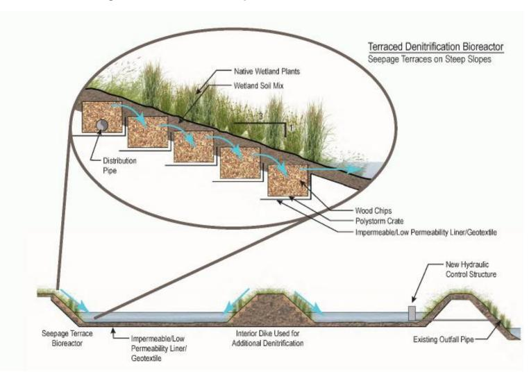
Figure C-2. Overview of Proposed Treatment Wetland Process
