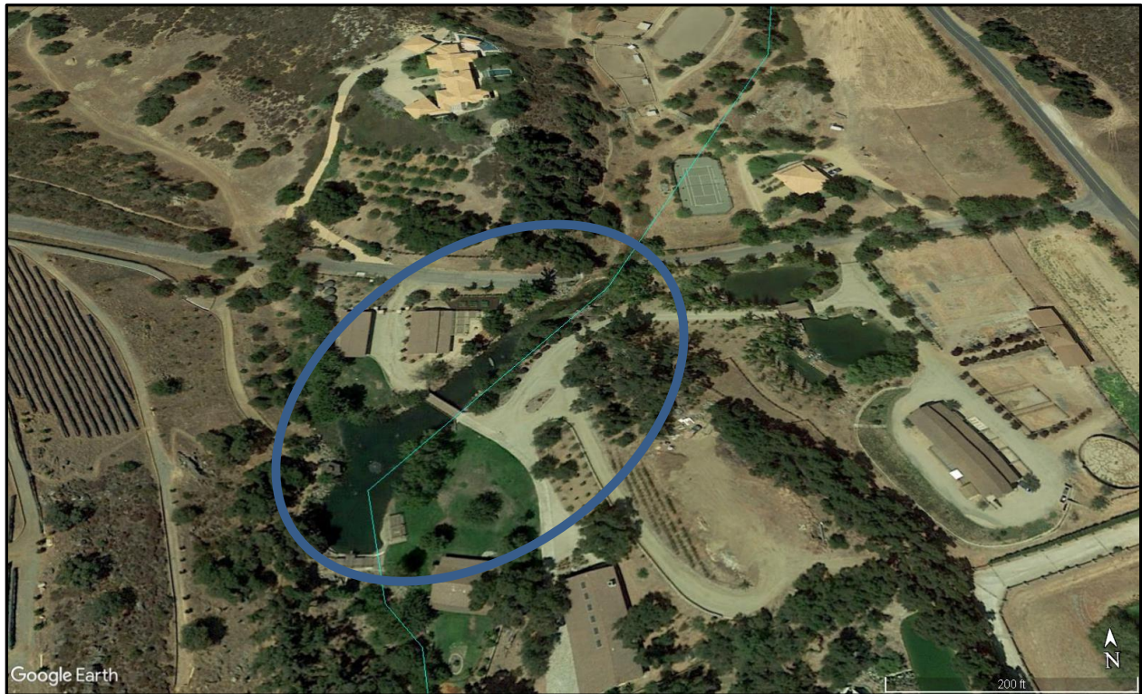
Figure 10. Example of Pond (circled) in the Upper San Mateo Creek Watershed. This pond is constructed in-line with the stream, which allows any stocked non-native species to move downstream during high flow events (photo: Google Earth).
