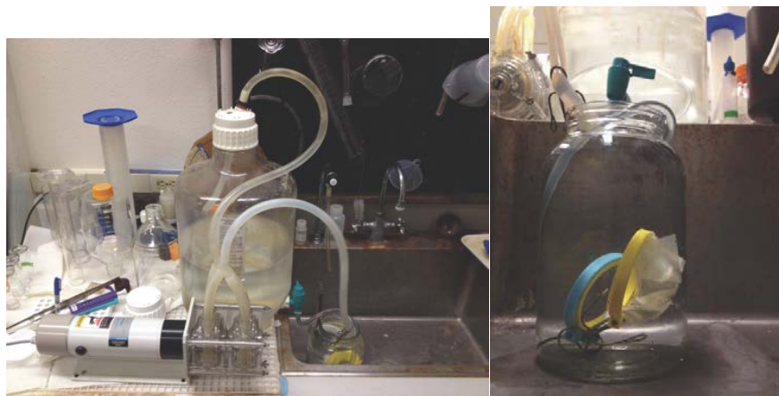
Figure 2. Laboratory setup for the flow-through testing of SPATT. Left photo shows the carboy, receiving container, and pump. Right photo shows SPATT (in colored embroidery hoops) within the receiving container.
