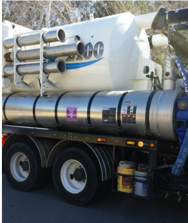
Vactor Truck for Sewer Flushing
