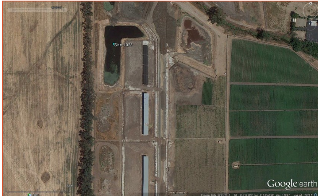
Figure 2. Example of a livestock waste pond (Table 2). The nearby rectangular metal roof structures that house animals are good identifiers of these systems. While these ponds should be excluded, abandoned stock ponds created to water livestock by damming seasonal streams in natural areas (not shown) are often included in depressional wetland surveys.
