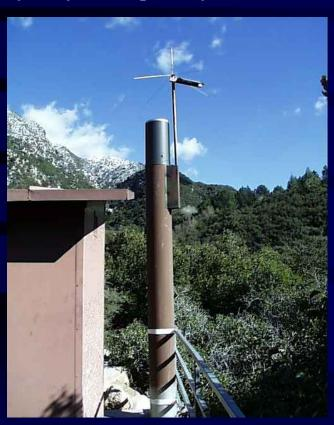
An outflow recorder is used to measure the amount of surface runoff at a point of observation.
