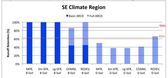
Figure 5a. Percentage of Runoff Retained Relative to Standards 1 (85<sup>th</sup> Percentile, 24-hour precipitation event) and 2 (95<sup>th</sup> Percentile event) for Southeast Climate Region
