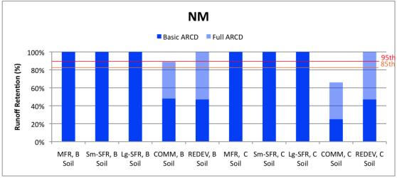
Figure 5c. Percentage of Runoff Retained Relative to Standards 1 (85<sup>th</sup> Percentile, 24-hour precipitation event) and 2 (95<sup>th</sup> Percentile event) for Northeast-Midwest Region
