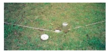
Figure 3. Tube-type lawn sampler (site 2).
