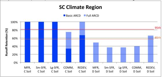
Figure 5b. Percentage of Runoff Retained Relative to Standards 1 (85<sup>th</sup> Percentile, 24-hour precipitation event) and 2 (95<sup>th</sup> Percentile event) for South Central Climate Region
