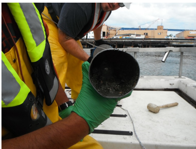
Sediment Core Plug from Station SD-N-C-16-D (May 18, 2015)
