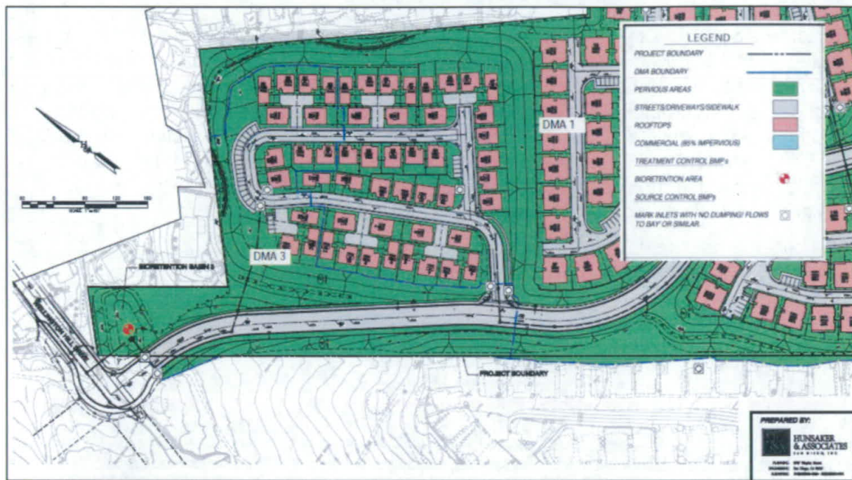
Figure 5: DMA Map for Settler's Point SWPPP showing off-site road knuckle connection to Wellington Hill Drive.
