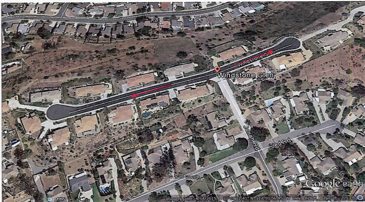
Photo 3(a): Google earth aerial view of Falcon Crest PDP on Windstone Glen Road. Stormwater flows in two directions toward the street ends.
