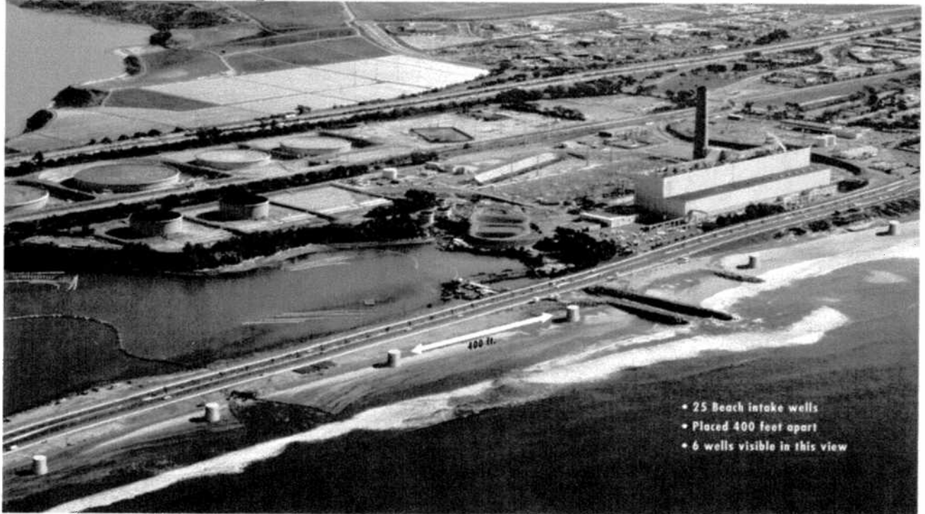
Figure 4-3 – Pump Stations with Horizontal Intakes
