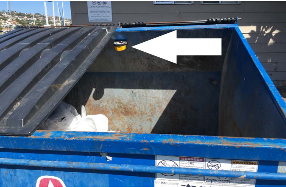
Ultrasonic sensors that detect receptacle fullness on an hourly basis
