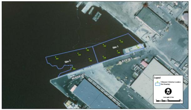
*Figure F-6. 2002 dredge area and sample locations at the Tenth Avenue Marine Terminal* Source: AMEC Earth & Environmental, Inc. (2002)
