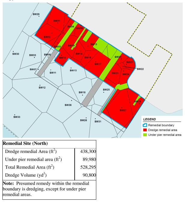
Attachment 3. Remedial Footprint Based on Sediment Management Units for BAE Shipyard
