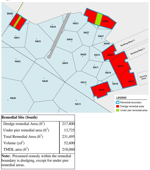
Attachment 4. Remedial Footprint Based on Sediment Management Units for NASSCO Shipyard
