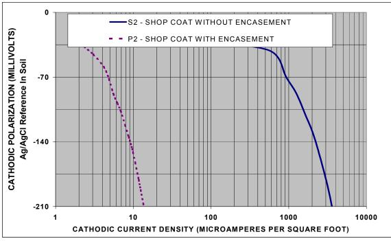
Figure 12 – Representative E-LogI Scans. Polyethylene encasement reduces cathodic current demand by ~99%.
