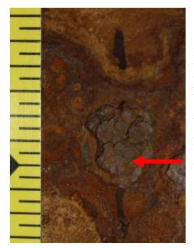
Figure 8 – Close up of corrosion product
