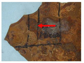
Figure 7 – Pipe specimen identified for metallographic analysis
