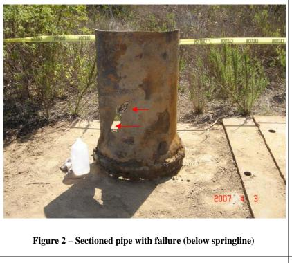
This is the section from above the spring line. This has not been cleaned, yet the band on the pipe adjacent to the bell can be seen. It is this band that delineates the taping of the PE encasement. There is no appreciable corrosion outside encasement or above the The four red springline. arrows locate the area of the corroded band.
