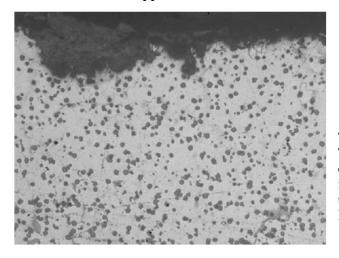
Micrograph of outside diameter surface Lower specimen. Etched 2% Nital Magnification 200X Cast Ductile Iron
