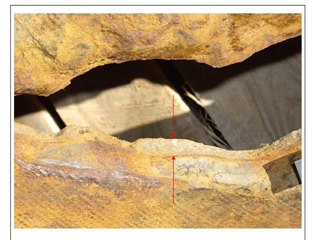
Figure 4 - Corrosion hole close-up
