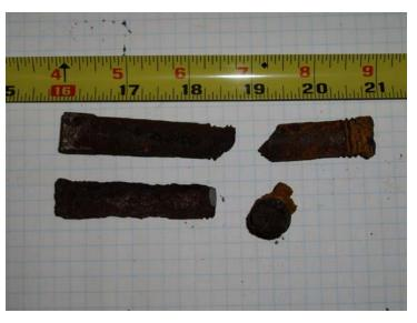
Figure 14 – Corrosion of fasteners
