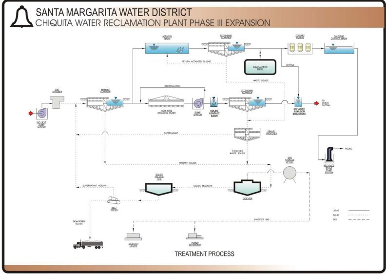
Attachment C – Flow Schematic
