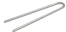
TLS6 Soil Staple On-surface applications should use one TLS6 for approximately every 4' of tubing, plus two on each tee, elbow or cross
