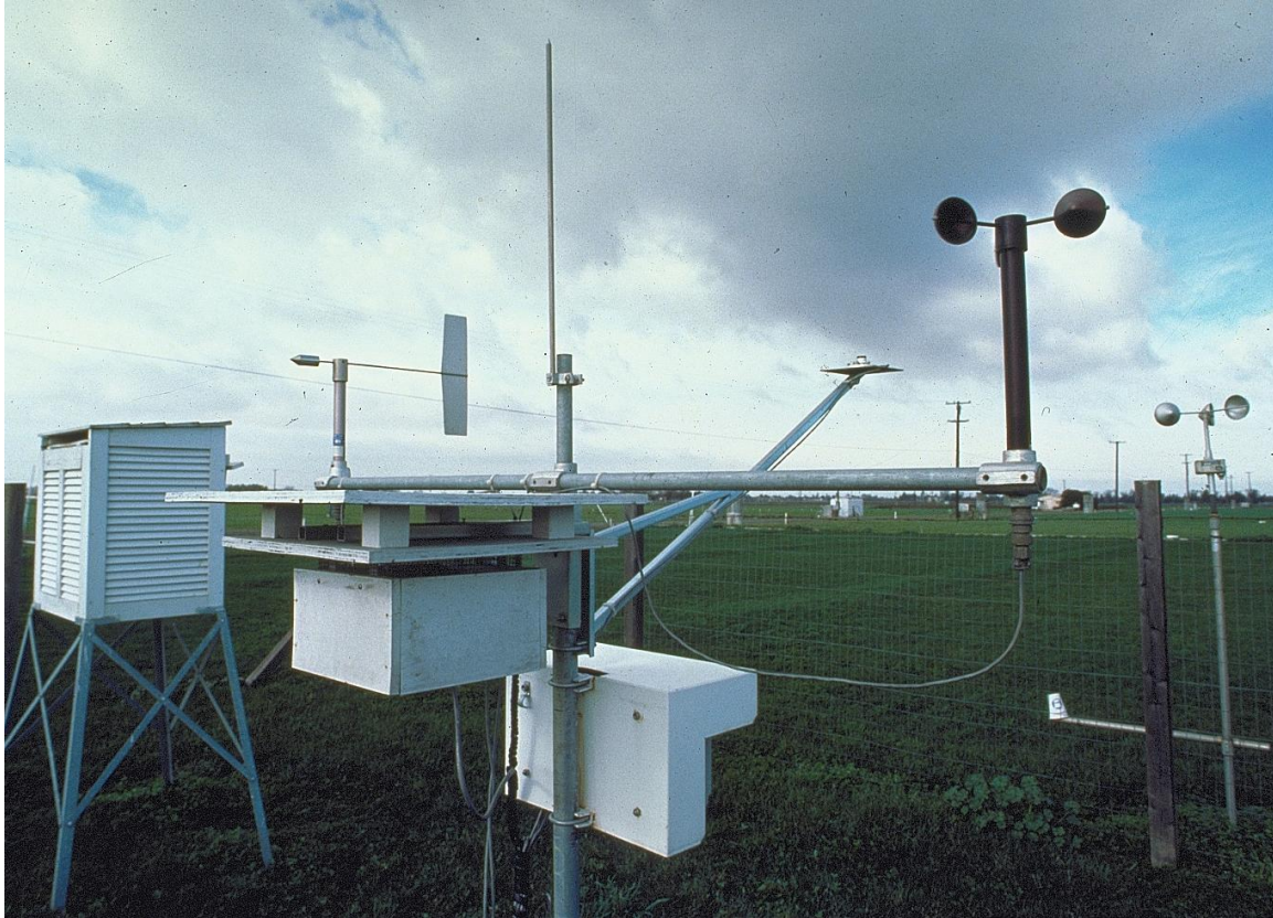
Photo VIII-1. A typical CIMIS weather station used to collect and transmit meteorological data used to calculate ET_0 .
