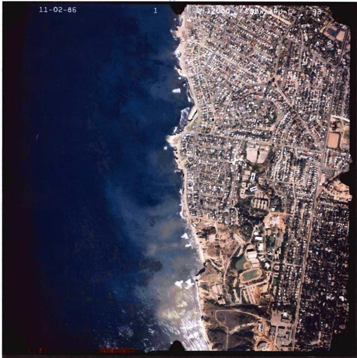
Figure 3. Aerial photograph taken November 2, 1986 of the SCNP area and turbid ocean waters. The turbidity of the ocean waters that is greatest off the southern areas of the SCNP Hillside Park, presumably due to erosion sediments that have been transported to the sea by runoff from SCNP and PLNU. Currents will move the turbidity plume north and southward along the coastline by a number of factors including: tides, wind and prevailing alongshore currents. This photograph is part of an aerial photographic time series for the California coastal zone that is available online, and is compiled by the California Coastal Records Project.
