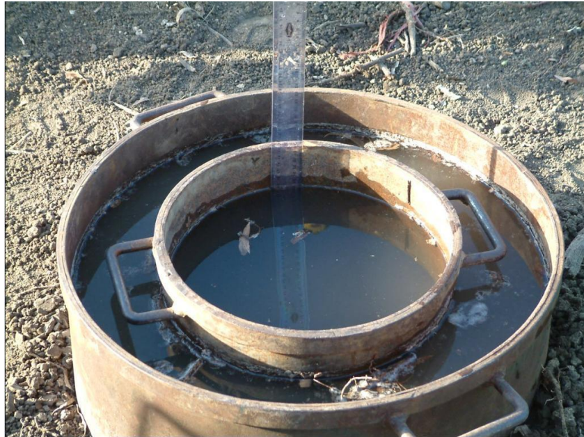
Figure VII.5. Photo of Simple Double Ring Infiltrometer
