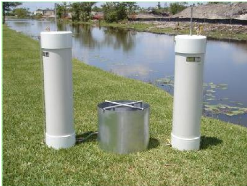
Figure VII.10. Double Ring Infiltrometer Set-up with Mariotte Tubes
