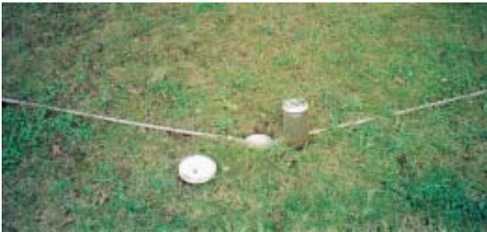
**Figure 3.** Tube-type lawn sampler (site 2).
