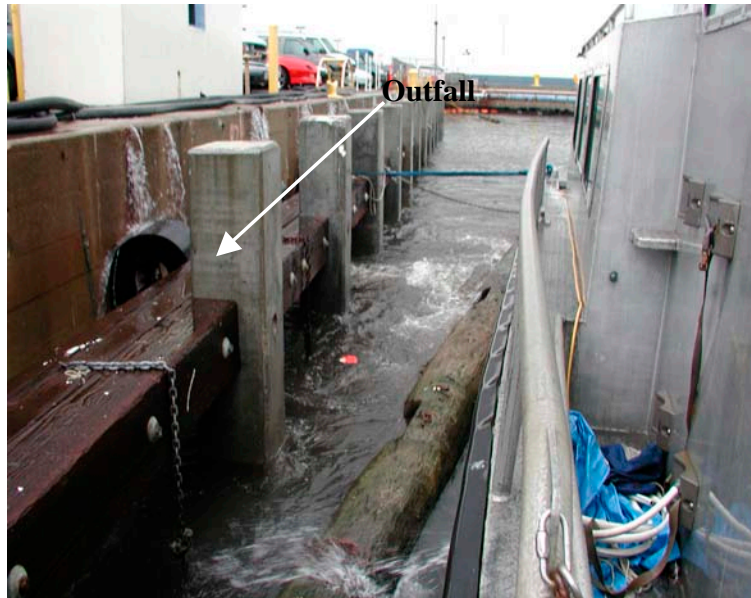
Figure 57. RV ECOS tied up along Naval Station San Diego quay wall outside outfall 14 during the special floating laboratory bioassay conducted in October 2004. The sensors and pump intake were ~ 15 feet away from the outfall. Note sheet runoff over quay wall.
