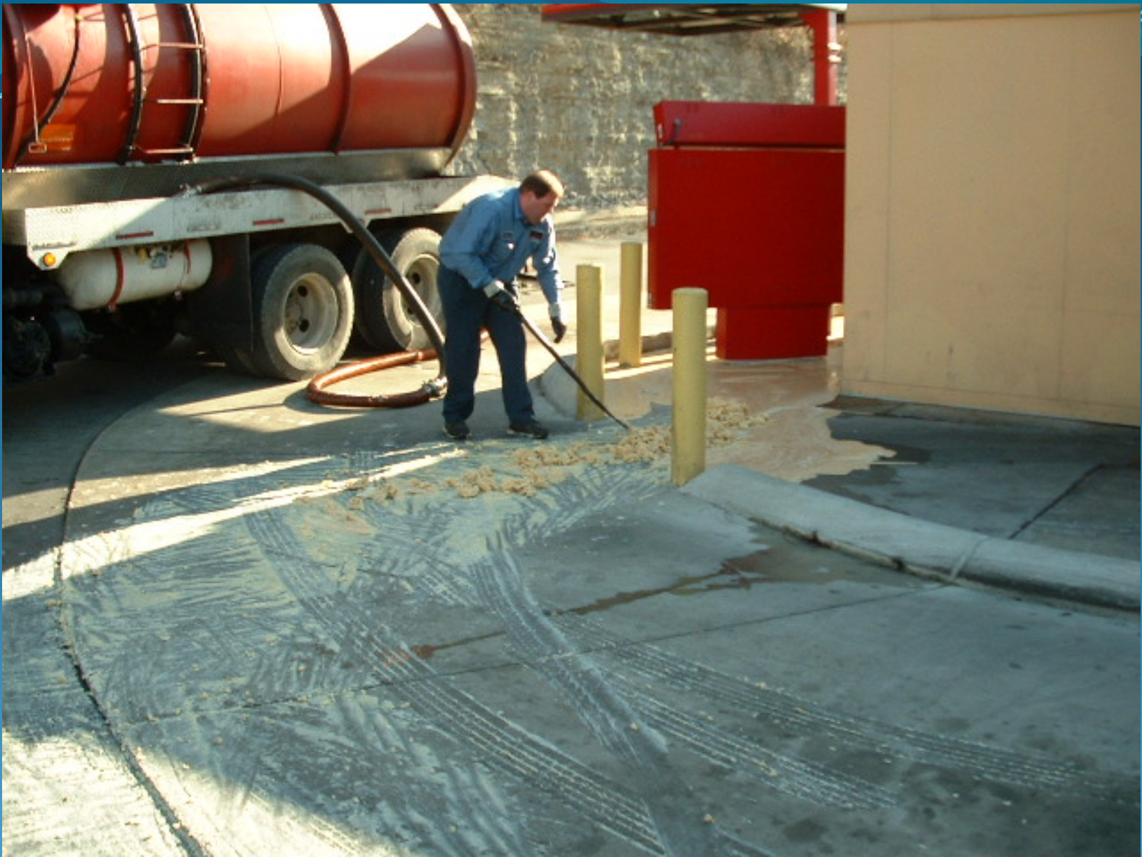
Automated grease recycle container overflow due to faulty level indicators
