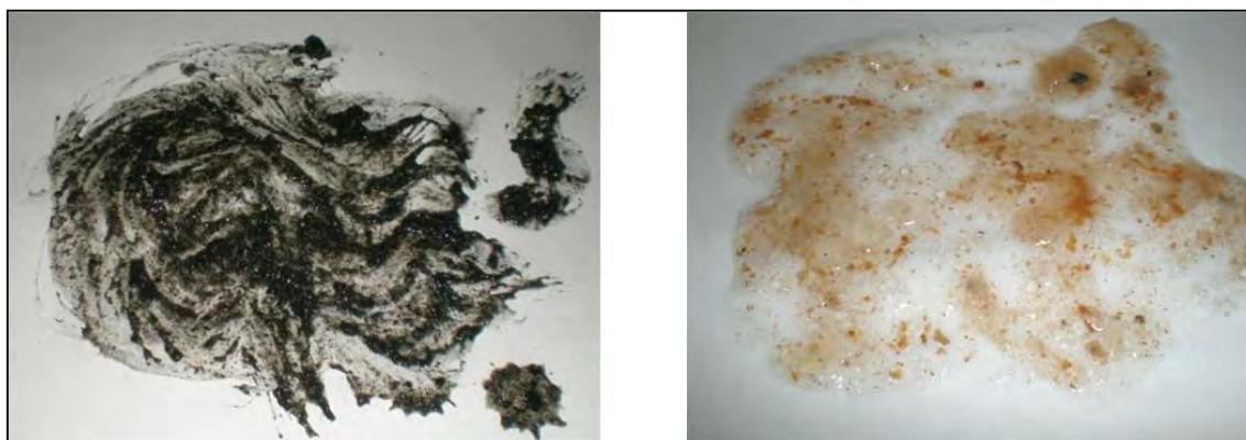
Photograph 1. Mineral and Biological Fouling Deposits shown on the left and right, respectively
