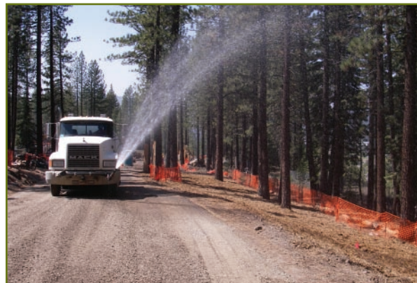
Highly adjustable fire hose nozzles can be attached to water trucks to produce a wide range of spray patterns and flow rates ideal for irrigation applications. Many water trucks that are equipped for dust control applications actually displace mulch and create erosion when used for irrigation.
