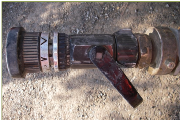
Highly adjustable fire hose nozzles can be attached to water trucks to produce a wide range of spray patterns and flow rates ideal for irrigation applications. Many water trucks that are equipped for dust control applications actually displace mulch and create erosion when used for irrigation.
