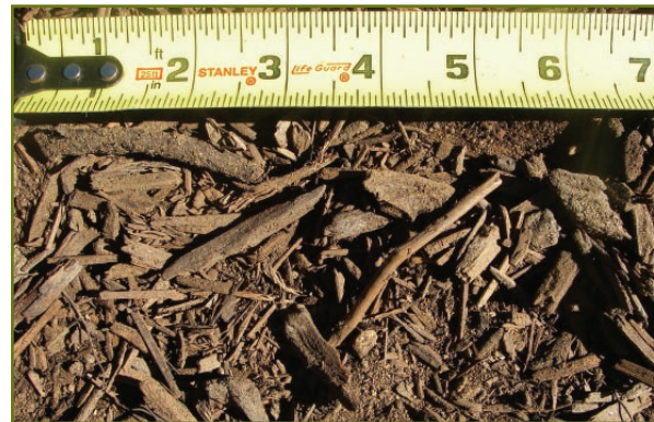
Coarse-textured compost blend – 50% coarse overs (3/8" – 3"), 50% fines (< 3/8")
