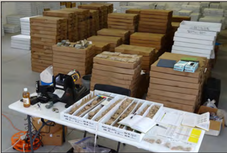
Figure 3. Hand-held X-ray fluorescence (XRF) instrument used to measure concentrations of up to 28 elements (including chromium) in rock, alluvium, and core material from Pacific Gas and Electric (PG&E) monitoring wells, Hinkley, California, March 2015 (core material archived by PG&E in background).
