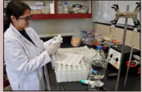
Figure 4. Preparation of sequential chemical extractions from alluvium and core material, Hinkley, California, June 2015.
