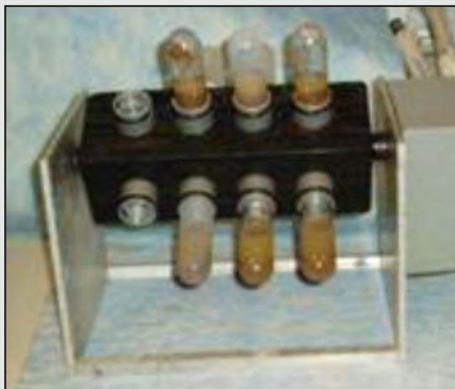
Figure 13. Experimental microcosms used to evaluate the potential reoxidation of trace elements over time.
