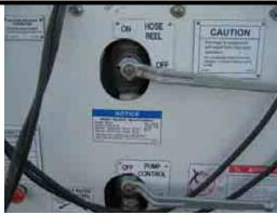
3f. Controls for water system pump control for Handgun, washout and Jetter hose.
