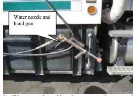
9a. Water nozzle and hand gun secured onto truck
