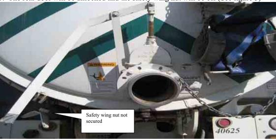
Figure 3: Truck with rear door unlocked & no safety wing nut
