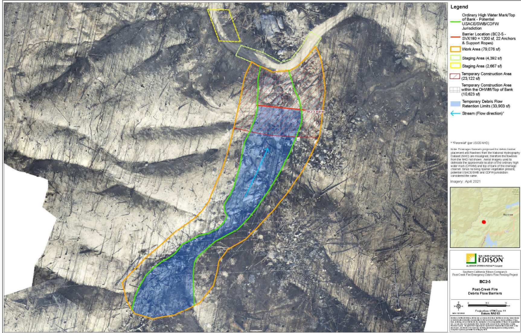
Figure 3: BC2-5 Work Area and Impacts
