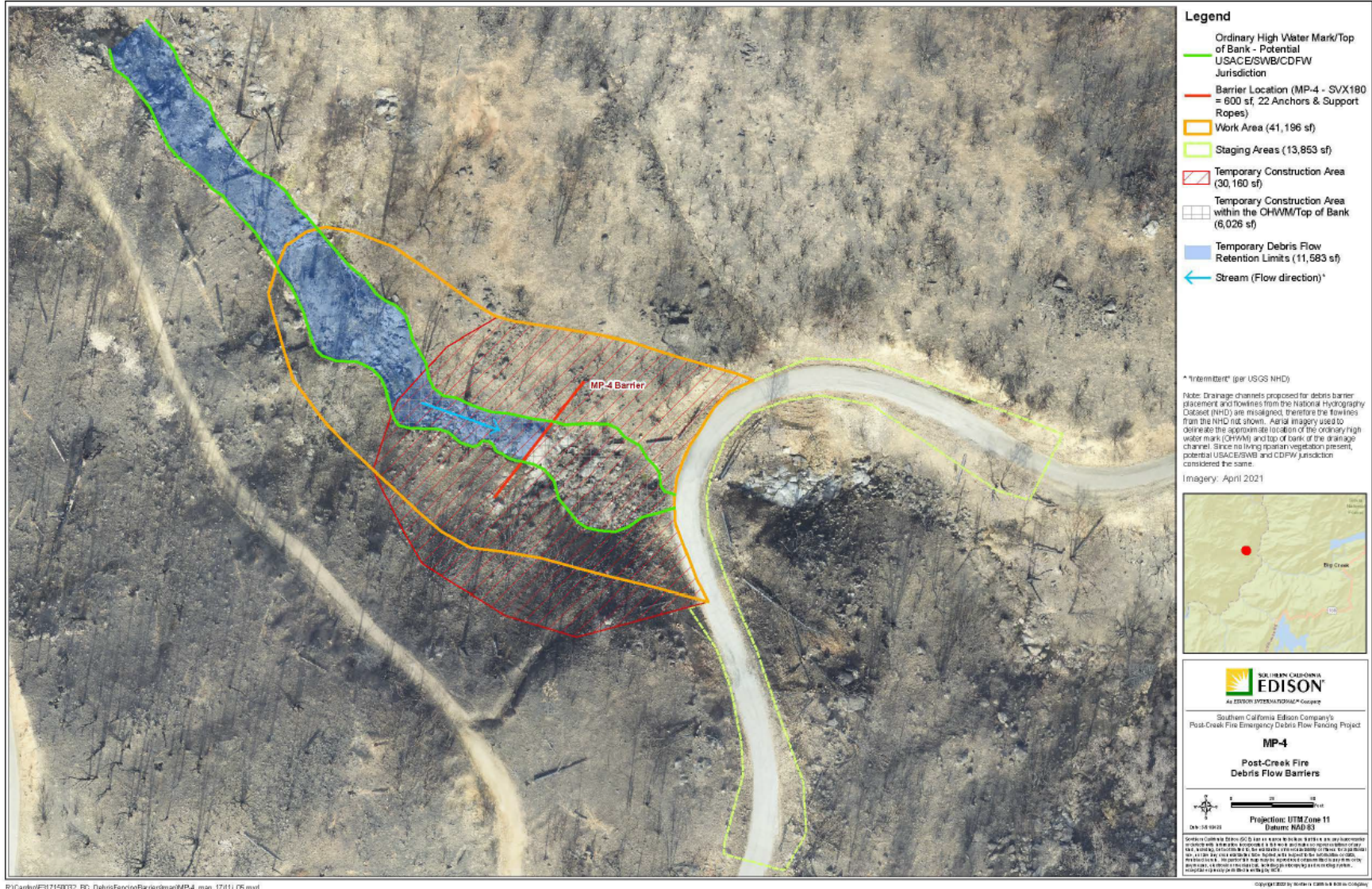
Figure 7: MP-4 Work Area and Impacts
