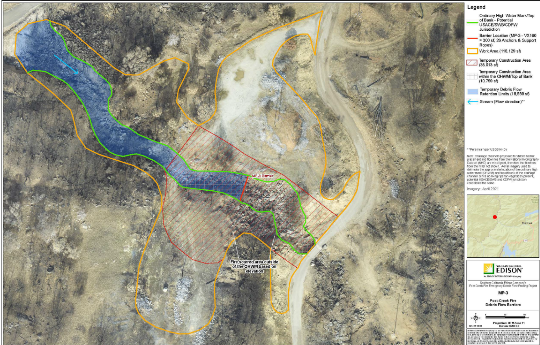
Figure 5: MP-3 Work Area and Impacts
