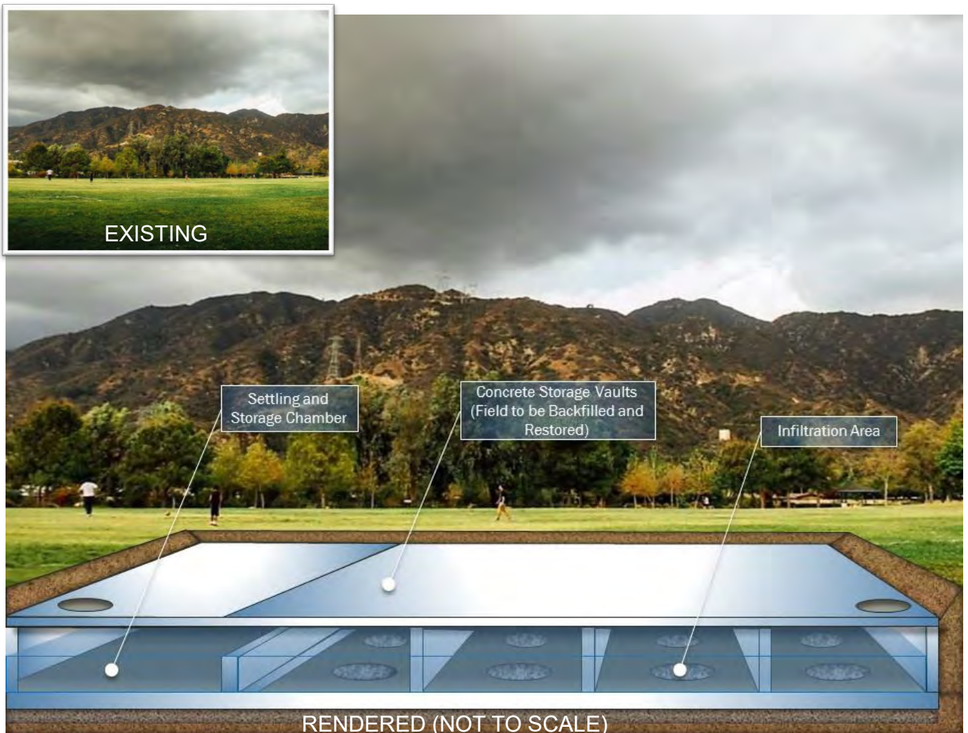
Figure 7. Rendering of Proposed Subsurface Structure at Encanto Park
