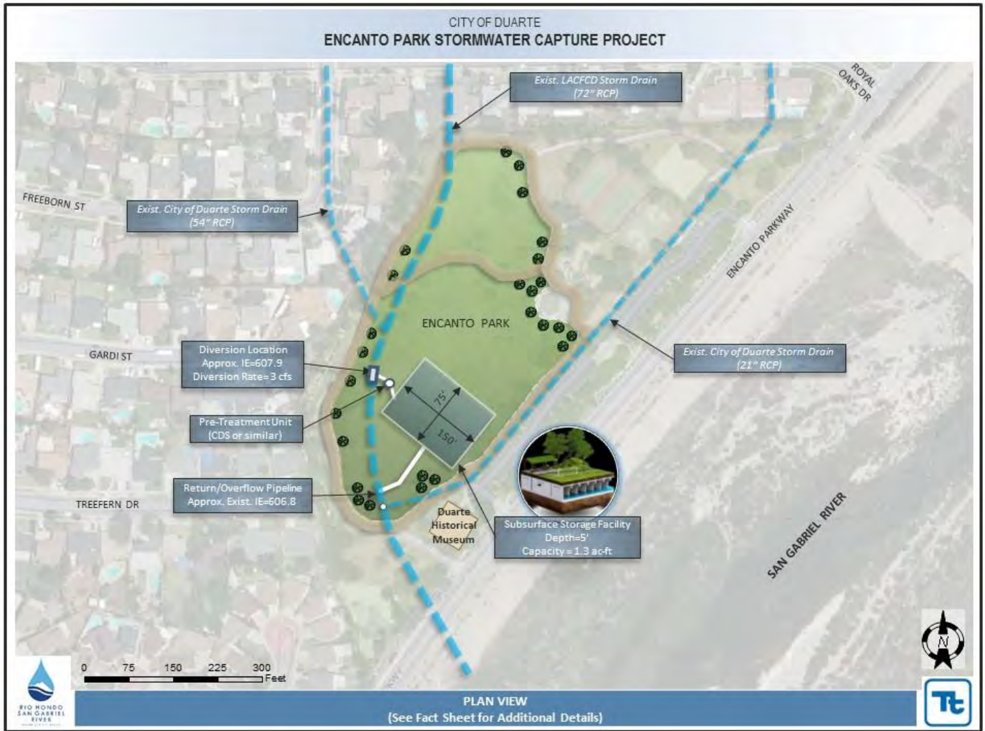
Figure 19. Encanto Park Stormwater Capture Project Site Layout
