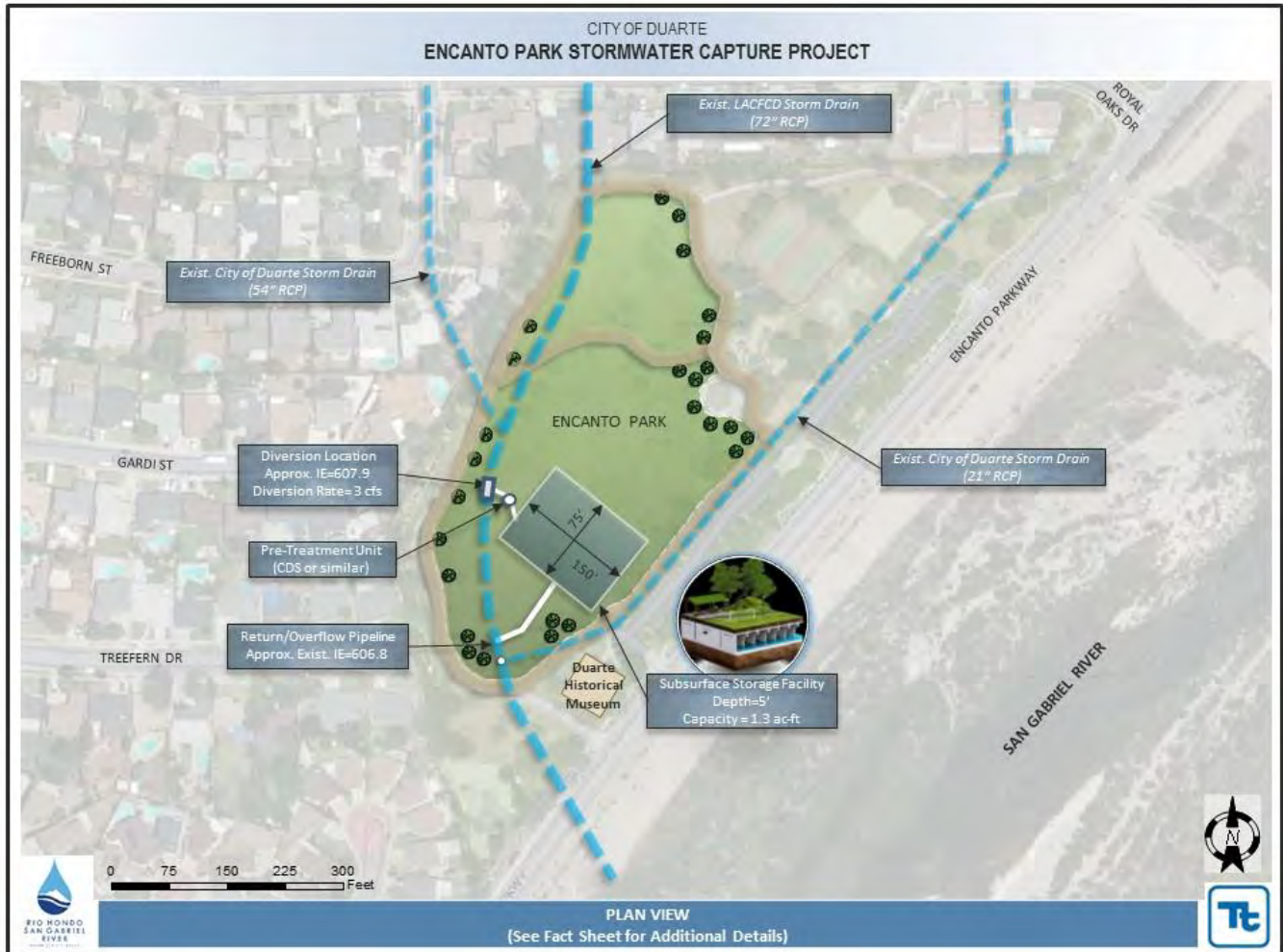
Figure 8. Encanto Park Stormwater Capture Project Site Layout
