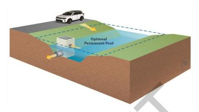
Figure 3-10: Wet detention basin schematic
