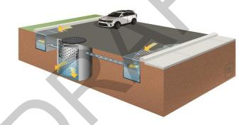
Figure 3-5: Drywell schematic
