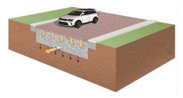
Figure 3-6: Porous pavement schematic
