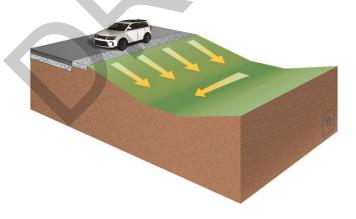
Figure 3-9: Vegetated swale schematic
