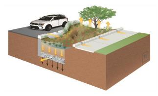
Figure 3-8: Bioretention with Underdrains schematic
