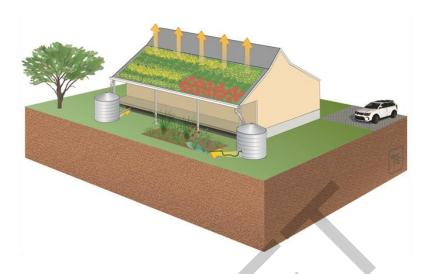
Figure 3-13: Above ground cisterns schematic
