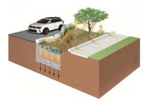
Figure 3-4: Bioretention without underdrain schematic
