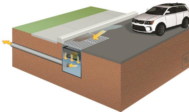
Figure 3-12: Pre-treatment BMP schematic
