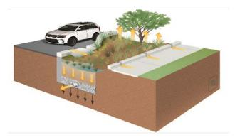
Figure 3-8: Bioretention with Underdrains schematic
