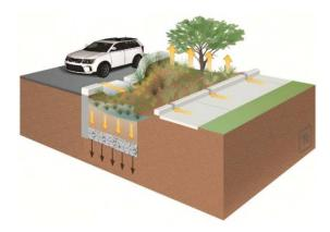
Figure 3-4: Bioretention without underdrain schematic
