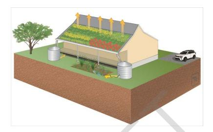
Figure 3-13: Above ground cisterns schematic
