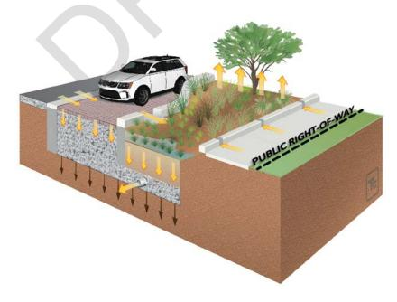
Figure 3-18: Right-of-way BMP schematic
