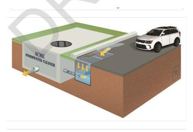
Figure 3-14: Underground detention schematic
