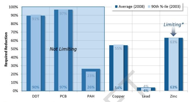
\* Organics managed through sediment and associated metals reductions. Organic load reductions above influenced by assigned concentrations at half the MDLs (monitoring data below MDLs), and therefore are suspect and not considered limiting.
