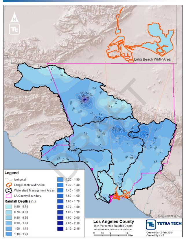
Figure 5-2. Rainfall depths associated with the 85<sup>th</sup> percentile, 24-hour storm.
