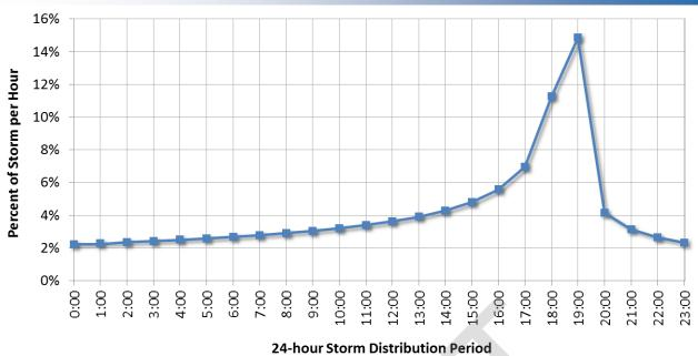
Figure 5-3. Temporal Distribution for 85th Percentile 24-hour Storm for LSPC Simulation.
