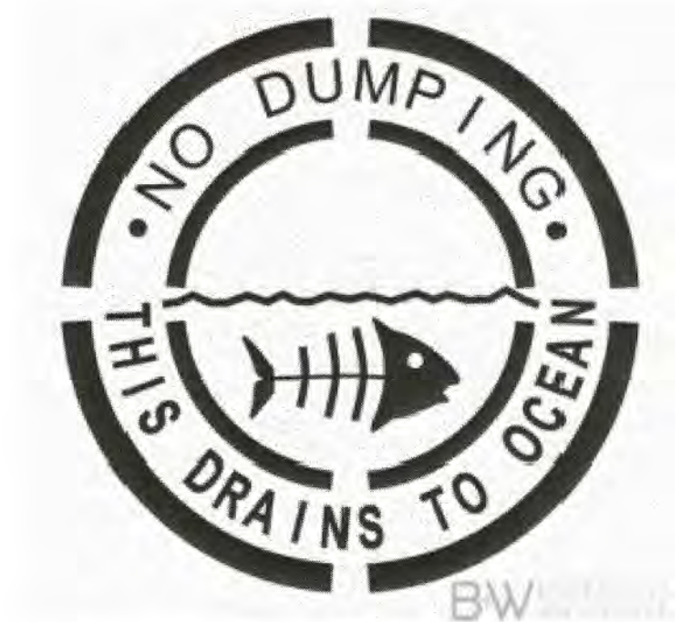
CATCH BASIN STENCILING DETAIL
