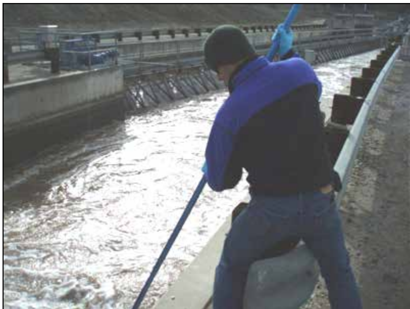
Figure 9-7. Grab Sampling Using Extended-Reach Swing Sampler
