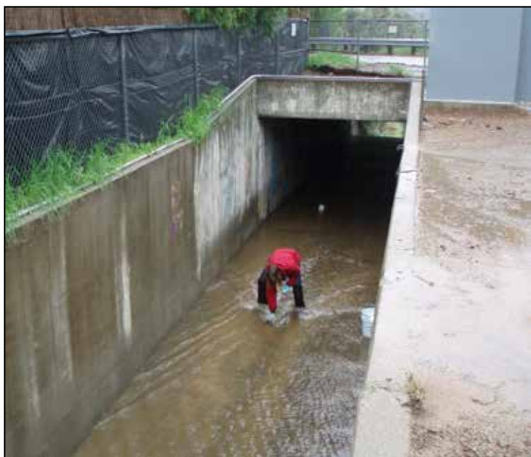
Figure 9-9-6. Grab Sampling at Mid-Stream, Mid-Depth
