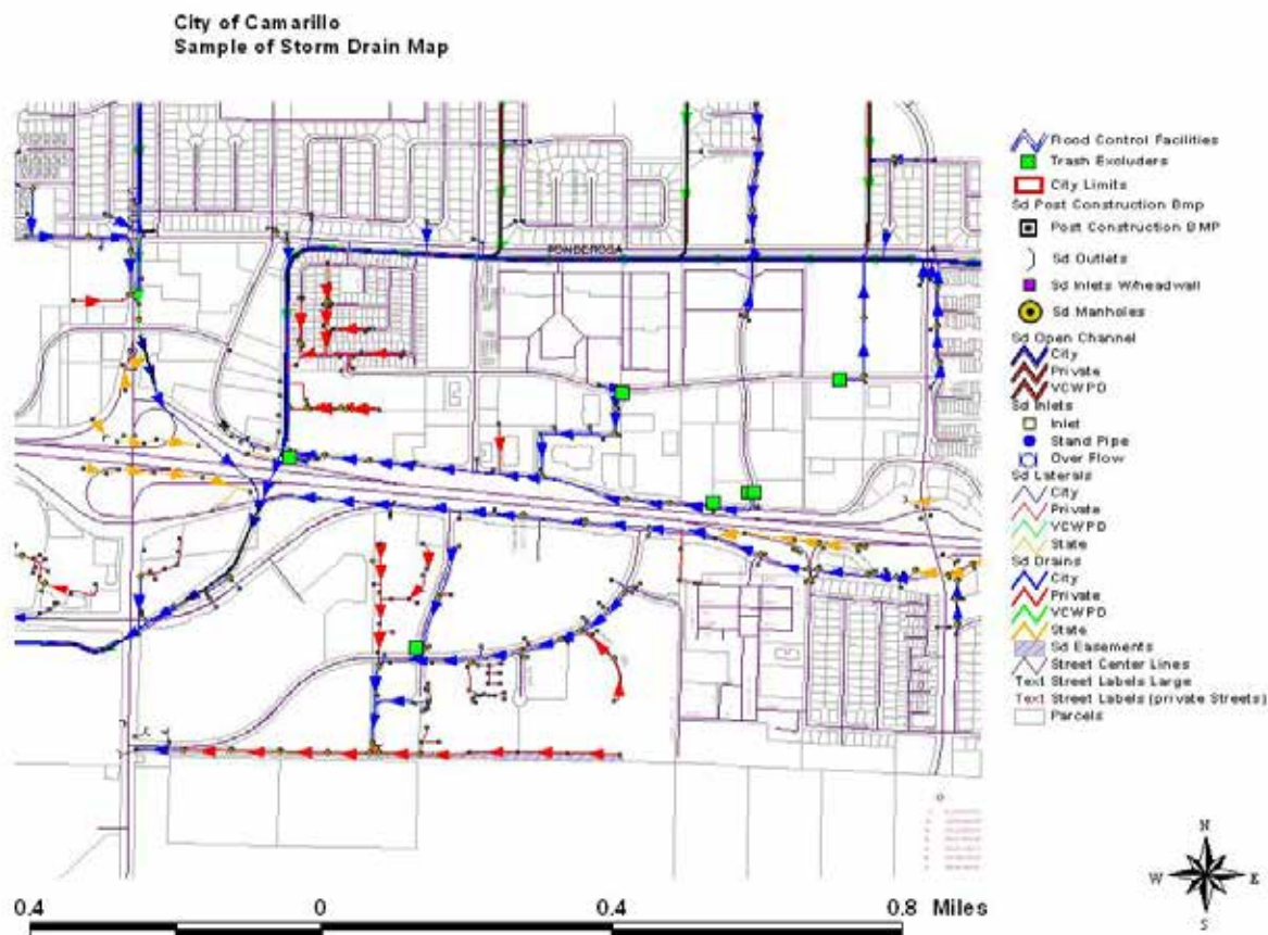
Figure 7-3 Example of Storm Drain Map
