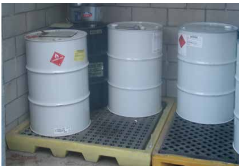
Materials stored with secondary containment
