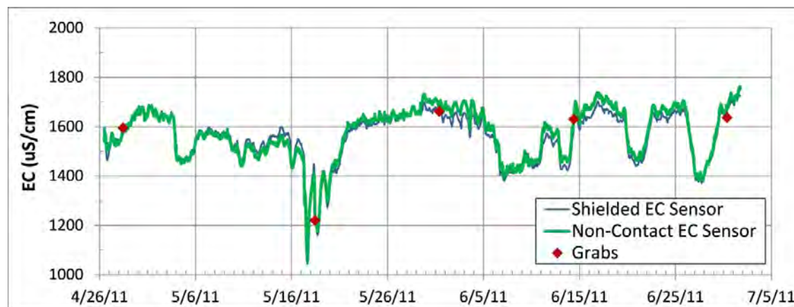
Figure 12. Comparison of continuous (5-min) EC sensor data from April 26-July 5, 2011 and intermittent grab samples for EC (field measurements using meter) at 03_UNIV.
