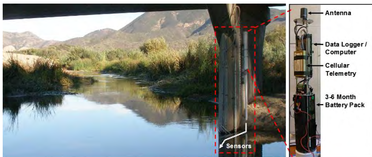
Figure 2. Left panel: Self-contained monitoring unit mounted to bridge at 03_UNIV site; Right panel; electronics with cover removed.
