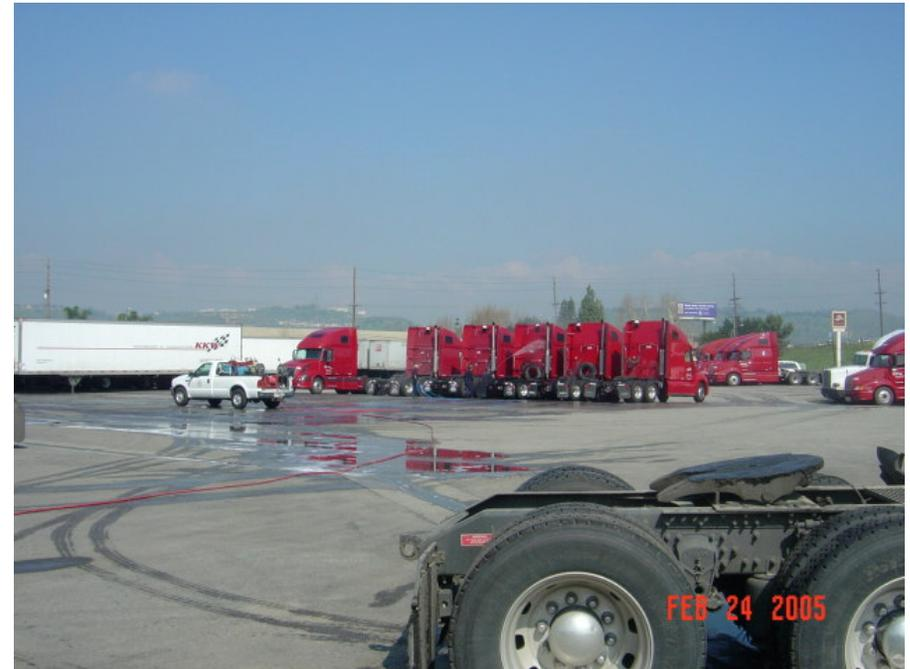
*Unauthorized non-storm water discharge because trucks were washed outside the wash rack by a vendor*
