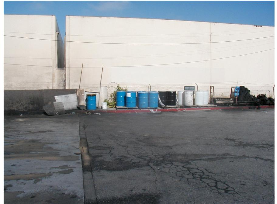
*Hazardous fluids should be stored within secondary containment. These uncontained drums contained grease, oil, antifreeze, and detergent.*
