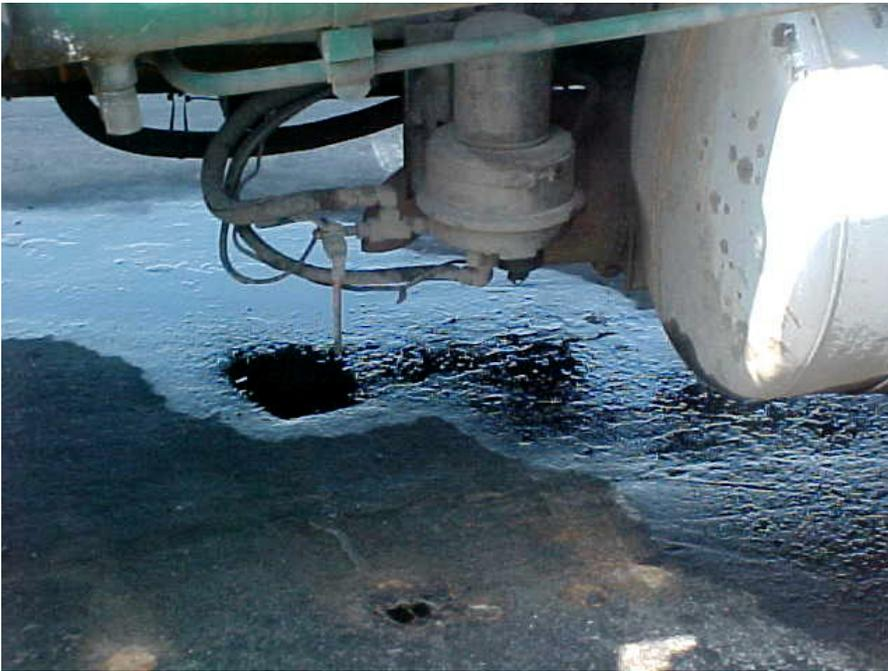
*Drip pans should be deployed beneath leaking vehicles*
