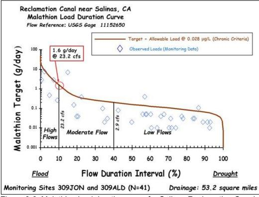
Figure 9-6. Malathion load duration curve for Salinas Reclamation Canal.
