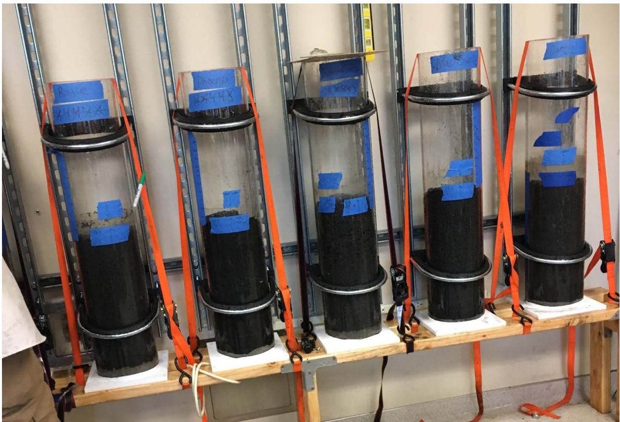
Figure 2. Column test setup at Sacramento State showing five of six columns
