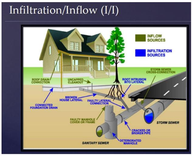
**Figure 7.7.** Example causes of inflow and infiltration. Source: <u>http://www.needhamma.gov/index.aspx?NID=320</u>
