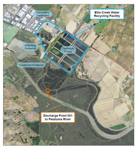
Figure 7.6. Ellis Creek Wastewater Treatment and Water Recycling Facility Map
