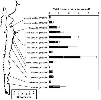
Figure 5. Total mercury in surface sediment (~0-5cm) 1999-2000 (Johnson et al., 2009).
