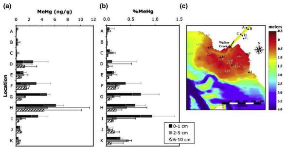
Figure 6. Methylmercury concentrations (a) and percent methylmercury (b) in the top 1, 2-5, and 6-10 cm of sediment cores. Results are averaged from three cores for each site taken at locations in the Walker Creek Delta area (c). After Johnson et al. (2009).
