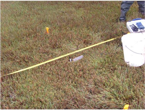
Figure 14.Sampling sediment at the Walker Creek marsh. Site was divided into 4<br/>quadrants (marked by orange stakes) in a circle with diameter of 2m<br/>(marked by measuring tape).
