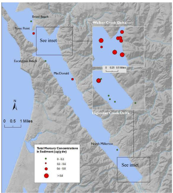
Figure 18. Total mercury in sediment. Each data point represents the average of two field replicates. Concentrations elevated above background ( $0.2 \mu g/g$  dry; Marshall 2006) are indicated by red, and were mostly isolated in the Walker Creek Delta area.
