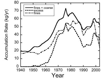
Figure 30. Estimated accumulation rate of mercury in the Walker Creek Delta (Johnson et al. 2009). Fines are defined as sediment <63  $\mu$ m, coarse sediments are >63  $\mu$ m, and excess mercury is defined as concentrations greater than 0.6  $\mu$ g/g.
