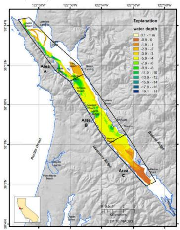
**Figure 9. Bathymetry of Tomales Bay (Anima, et al. 2008).** Note black outline indicates where bathymetry was measured, which does not include much of the Walker and Lagunitas Creek deltas.
