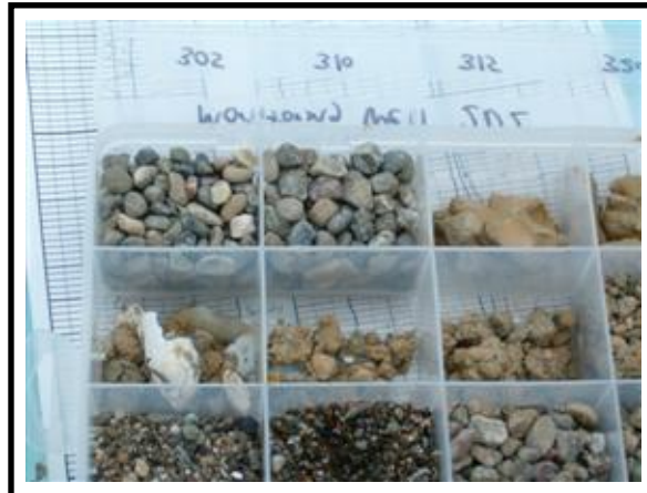
Gravels and sands (i.e., good aquifer materials) were encountered at the 300-foot depth. Samples were collected every 5 feet.
