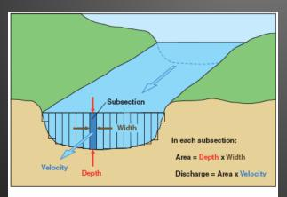
Current-meter discharge measurements are made by determining the discharge in each subsection of a channel cross section and summing the subsection discharges to obtain a total discharge.
