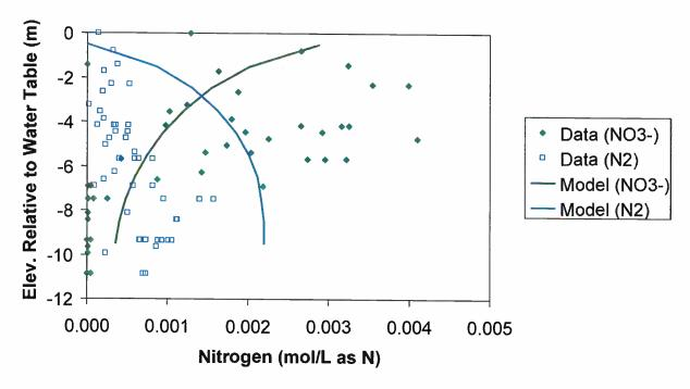
Figure 13. Simulation of denitrification associated with dairy wastewater percolation.
