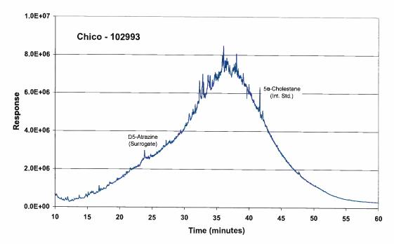
Figure 12. TIC of Chico sample 102993 showing the large amount of unresolved organic material present in this water sample. For scale, the internal standard in this sample represents 1  $\mu$ g/L.
