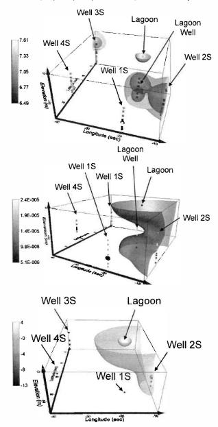
FIGURE 6. Distributions of pH (top), Ar (middle), and  $\delta^{13} C$  (bottom) in site groundwater, each consistent with lagoon seepage that may have impacted Well 2S at depths greater than 11 m. Isosurface values for pH correspond to 6.75, 6.8, and 7.3. The isosurface value for Ar corresponds to 3.6  $\times$  10<sup>-4</sup> mol/L. The isosurface values for  $\delta^{13} C$  correspond to -6.4 and 2.3 per mil.
