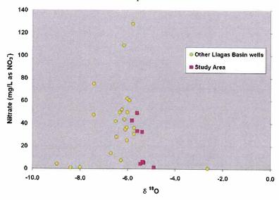
**Figure 17.** The ratio of nitrate versus stable isotope signatures of oxygen in wells from the region affected by wastewater irrigation (pink symbols) and in other shallow wells in the Llagas Basin (yellow symbols). Wastewater-influenced groundwater is shifted to more enriched isotopic values compared to ambient groundwater.
