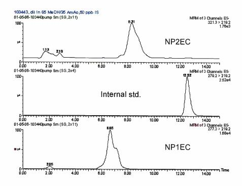
Figure 19. LC/MS/MS chromatogram of NP1EC (m/z 277 $\rightarrow$ 219) and NP2EC (m/z 321 $\rightarrow$ 219) in a Gilroy groundwater sample. The effective concentration of the internal standard (m/z 279 $\rightarrow$ 219) is 1 µg/L. The likely reason that the NP1EC and NP2EC peaks are broader than the internal standard peak (which is a labeled form of AP1EC) is that the former peaks represent mixtures of isomers whereas the internal standard peak represents a single compound only.
