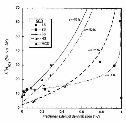
FIGURE 4. Nitrate  $\delta^{15}$ N values plotted against the fractional extent of denitrification (1 - f) based on excess N<sub>2</sub> and residual nitrate. Enrichment factors ( $\epsilon$ ) are calculated by fitting the Rayleigh fractionation equation to data from three multilevel well sites at KCD and wells at MCD.
