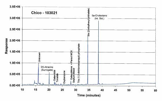
**Figure 14.** TIC of sample 103021, showing polycyclic musks, sunscreen compounds and tris (1,3-dichloroisopropyl) phosphate.
