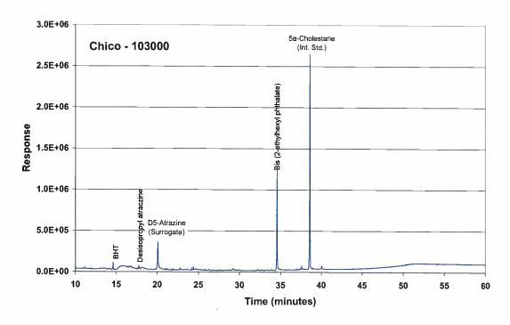
**Figure 13.** TIC of sample 103000, showing internal standard, surrogate compound, and desisopropyl atrazine (25 ng/L).
