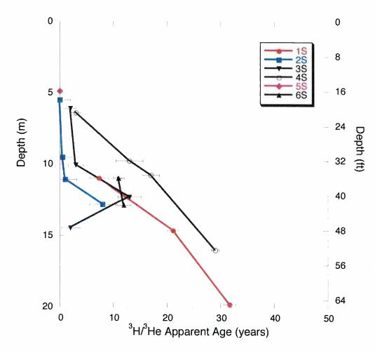
Figure S1. Groundwater  $^3H/^3He$  apparent ages from multilevel monitoring wells at KCD. Error bars show analytical error.
