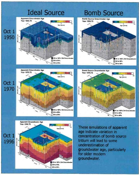
Figure 17. Simulation of apparent groundwater age at KCD1.
