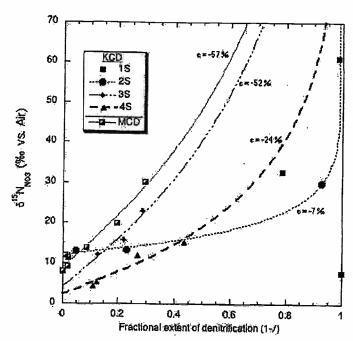
FIGURE 4. Nitrate  $\delta^{15}N$  values plotted against the fractional extent of denitrification (1 — f) based on excess  $N_2$  and residual nitrate. Enrichment factors ( $\epsilon$ ) are calculated by fitting the Rayleigh fractionation equation to data from three multilevel well sites at KCD and wells at MCD.
