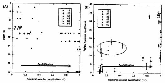
FIGURE 5. Sample depth (A) and  ${}^{3}H_{c}^{4}He$  apparent age (B) plotted against the tractional extent of denitrification (1 - f). Samples at two sites have experienced less denitrification than is typical for samples with  ${}^{3}H_{c}^{4}He$  apparent age >8 years (circled, see text).
