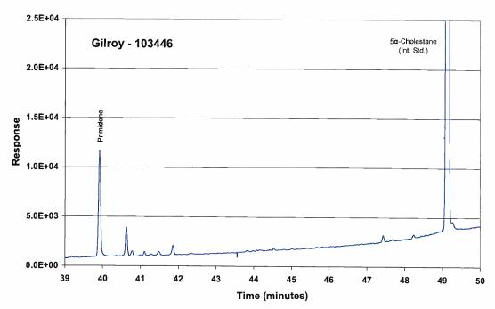
Figure 21. TIC of sample 103446, showing common plasticizer contaminants and primidone.
