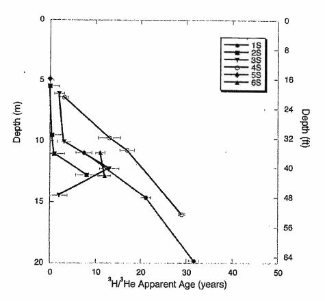
Figure S1. Groundwater <sup>3</sup>H/<sup>3</sup>He apparent ages from multilevel monitoring wells at KCD. Error bars show analytical error.
