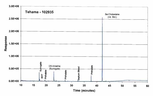
**Figure 7.** TIC of sample 102935. This GC/MS chromatogram is representative of the typical water extract from the Tehama study area.
