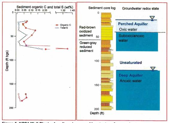
Figure 5. KCD1 Well Cluster 1 sediment composition, texture & groundwater oxidation state
