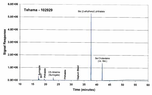
**Figure 8.** TIC of sample 102929, showing an unusually large amount of bis (2-ethylhexyl) phthalate.
