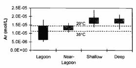
FIGURE 5. Thermodynamic saturation indices for calcite in site water samples, calculated with PHREEQC (left) and Ar concentrations and solubility (22) (right). The box-whisker marks correspond to the minimum, maximum, median, lower quartile, and upper quartile values for each group. Deep samples exclude groundwater samples from Well 2S.
