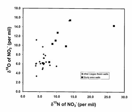
Figure 18. Nitrogen and oxygen isotope ratios in nitrate show a pattern characteristic of denitrification in samples influenced by recharge of wastewater.
