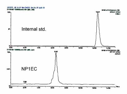
Figure 28. LC/MS/MS chromatogram of AP1EC (m/z 277 $\rightarrow$ 219) in a Livermore golf course groundwater sample. The effective concentration of the internal standard (m/z 279 $\rightarrow$ 219) is 1  $\mu$ g/L.
