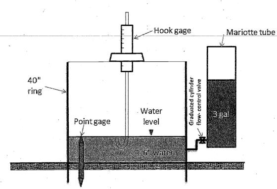
Figure VII.3. Single Ring Infiltrometer Setup with Mariotte Tube
