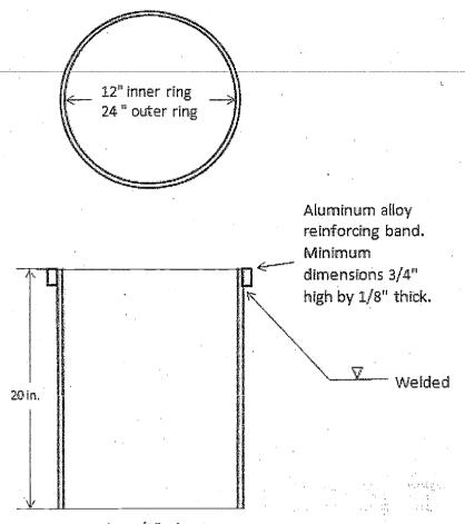
Figure VII.8. Double Ring Infiltrometer Construction
