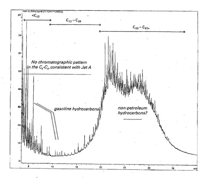
Figure 4. USCG Marine Safety Laboratory gas chromatogram of sample "CP-MW-2 (Source)". Preponderance of chromatographic signal is in the C<sub>9</sub>-C<sub>12</sub> range, and consistent in character with automotive gasoline. Small cluster of chromatographic peaks in the ~C25~C28 range are not readily recognized as a petroleum product; it is likely that these are hydrocarbons of some non-petroleum origin. There is no chromatographic evidence for the
