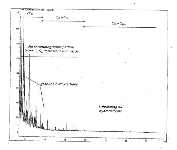
Figure 3. USCG Marine Safety Laboratory gas chromatogram of sample "CAH-MW-1 (Source)". Preponderance of chromatographic signal is in the C<sub>20</sub>-C<sub>35+</sub> range (consistent in character with complex mixture of lubricating oil), and C<sub>9</sub>-C<sub>12</sub> hydrocarbons consistent with automotive gasoline. There is no chromatographic evidence for the presence of Jet A. -
