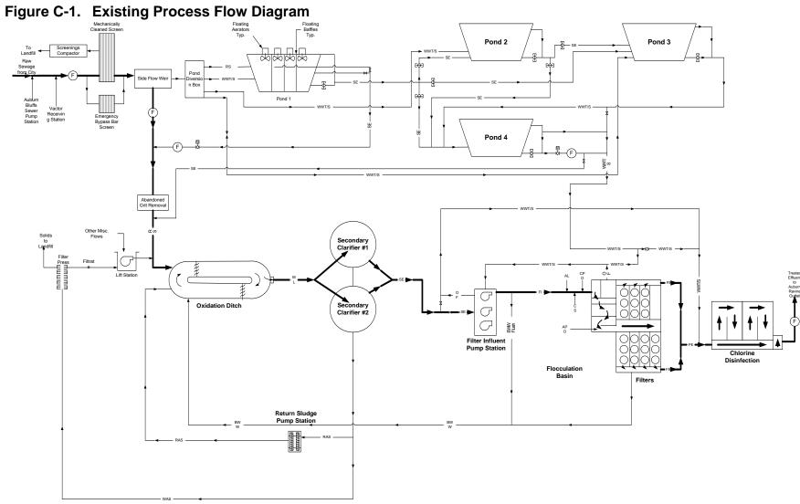
Pond 3 Raw Sewage 1.67 mgd ADWF <9 mgd PWWF 1.67 mgd avg. Abandoned Grit Removal Ca(OH)<sub>2</sub> Secondary Clarifier #2 1.67 mgd avg 3.5 mgd peak Secondary Oxidation Ditch Filter Influen Pump Station Secondary Clarifier #3 Flocculation Return Sludge Pump Station 0.03 mgd WAS UV 1.67 mgd avg 6.1 mgd peak Chlorine Contact Chamber **UV Disinfection** (used for emergency storage)
